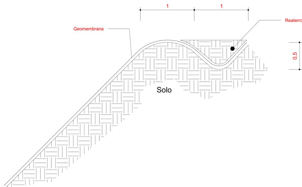
12 DETALHE - ANCORAGEM DA GEOMEMBRANA
